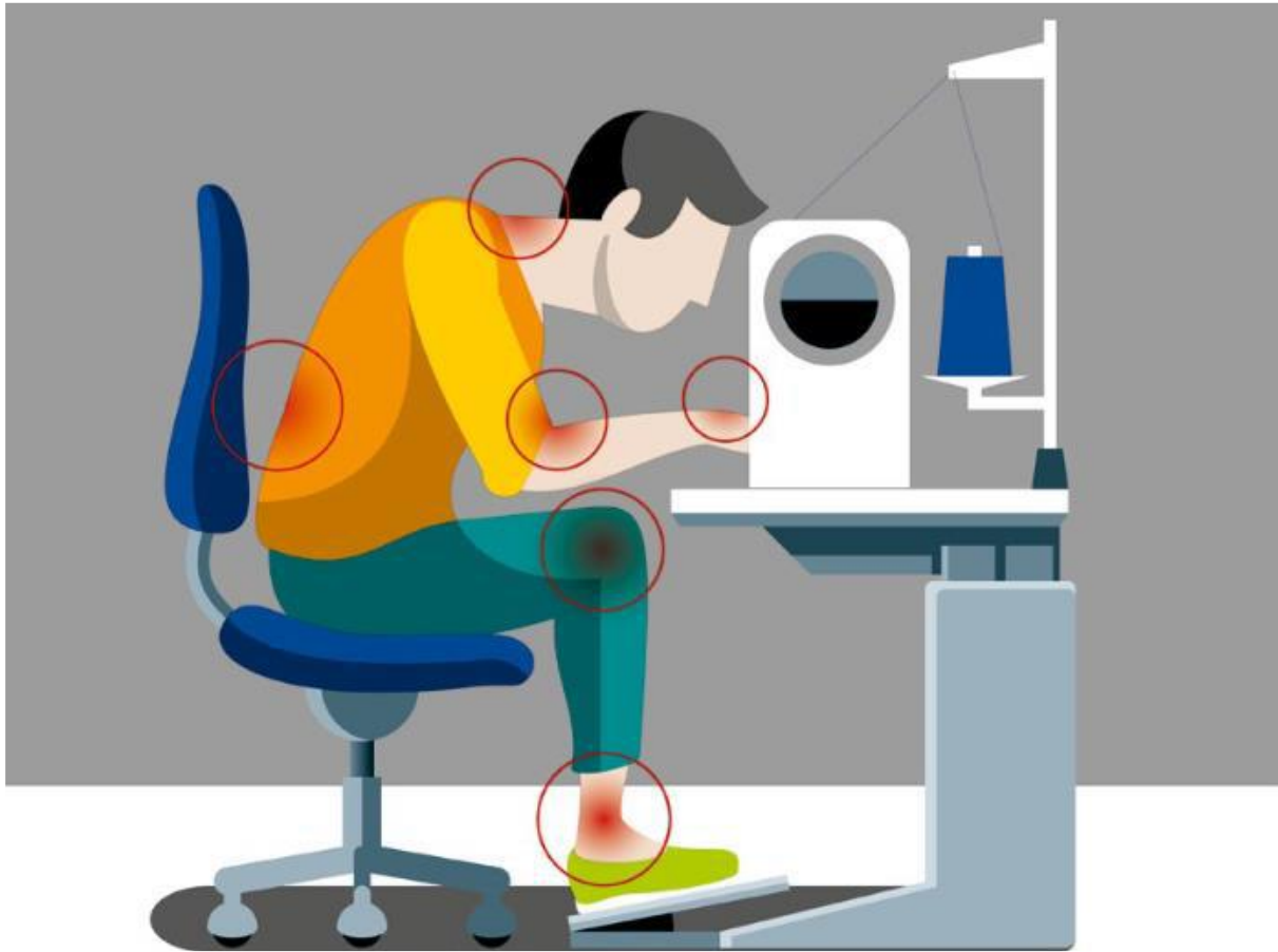
FIGURE: NON-ERGONOMIC SEWING WORKPLACE WITH IDENTIFICATION OF AREAS OF INCREASED HEALTH RISK. SOURCE: DGVU: ERGONOMICS AT SEWING WORKPLACES.142
